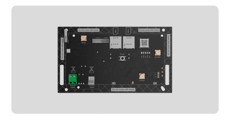
**Hub BP Jeweller (without casing)** is a wireless battery-powered control panel designed for installation in an Ajax casing. It supports photo verification. The hub connects to the Ajax Cloud server via two SIM cards (2G/3G/LTE) and has external antenna connectors for cellular, Jeweller, and Wings communication channels.
